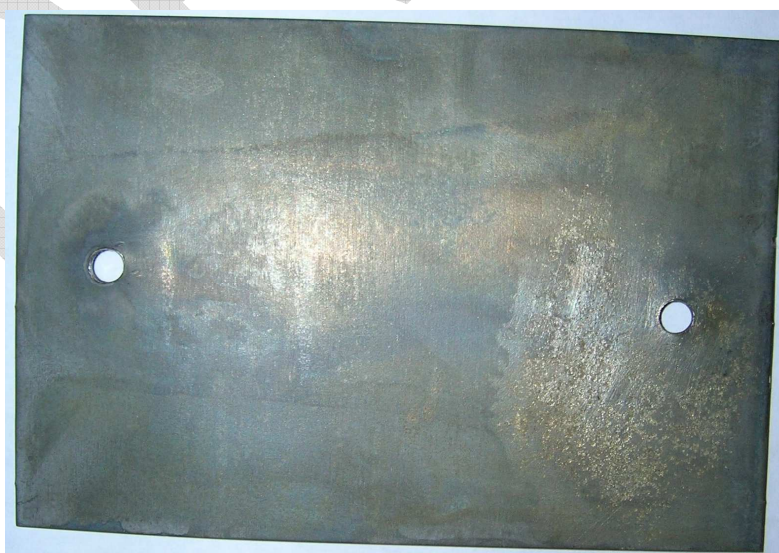
Figure 15 – Pitting of G90 specimen (zinc coating removed) after 12 months of exposure
