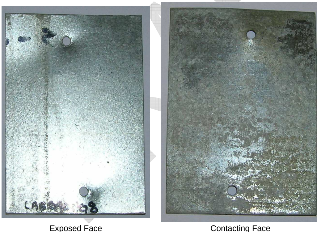
Figure 13 – Corrosion of exposed and contacting faces of a typical coupon specimen
