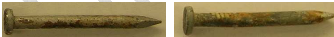
Hot galvanized nail Hot dipped galvanized nail Figure 16 – Corrosion of nails after 12 months of exposure (before cleaning)
