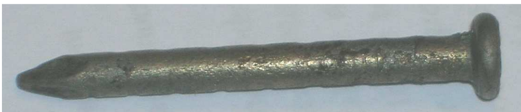
Figure 17 – Pitting of hot galvanized nail (zinc coating removed) after 12 months of exposure
