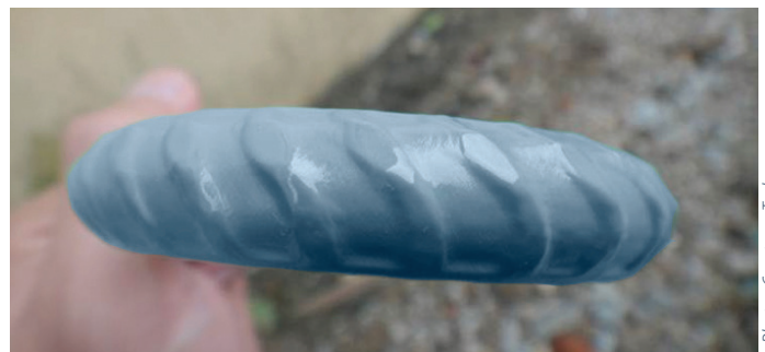
Laboratory produced 'BlueBar™' showing good bending and adhesion
