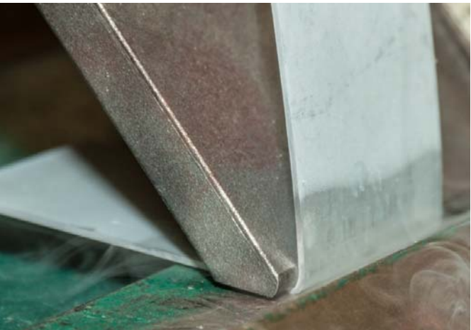
Fig. 29: Bend test at 90° for DP980.
